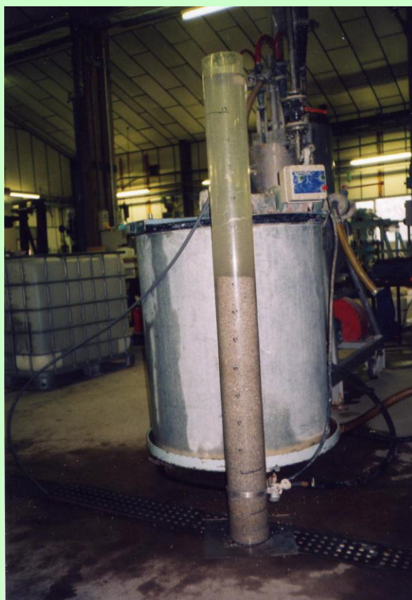
Figure 17. Perspex column used in packed bed experiments at WBB Minerals.
