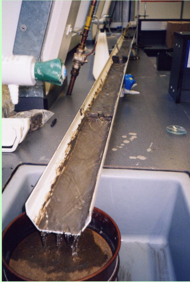
Figure 9. Indoor re-circulating flume showing clay bed.
