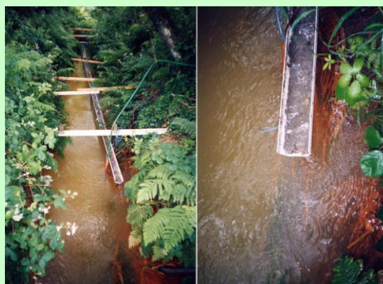
Figure 16. Experimental Trials of Clay Flume at Dolcoath Adit
